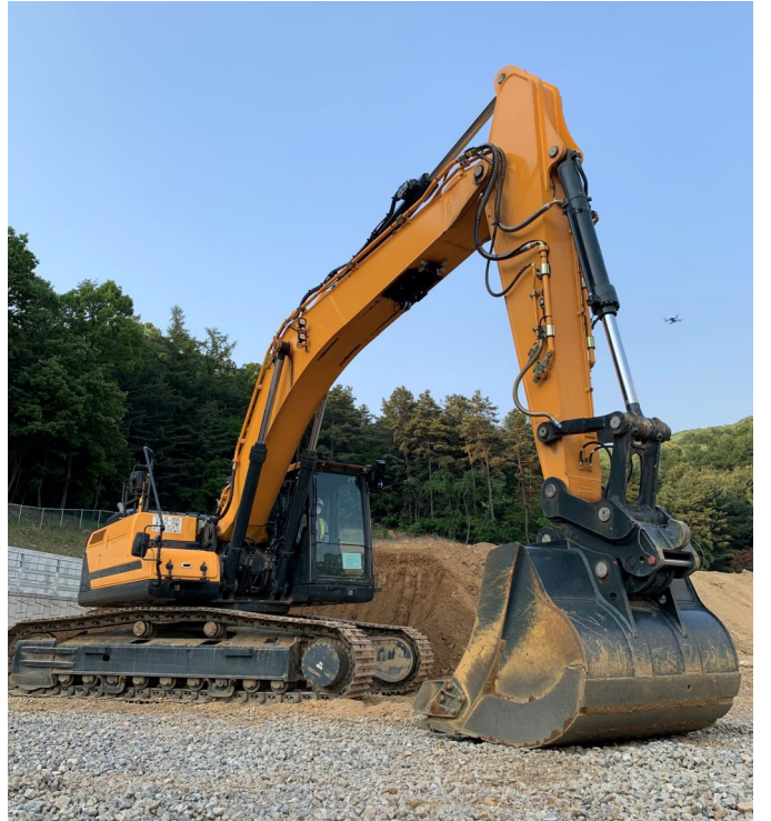
Fig. 1: The 30-ton hydraulic excavator hardware considered in this research. The proposed AES is capable of performing earthcutting and post-excitation inspection works fully autonomously using only onboard sensors.
