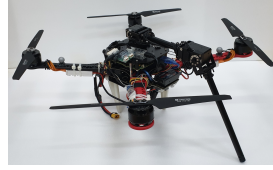
Fig. 1. Aerial manipulator prototype. Note that we do not assume a particular robotic arm configuration in dynamic modeling and control design.
