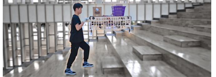
Fig. 1. Cargo transportation based on pHRI with the Palletrone mUAV. Human operators can load cargo onto the upper surface of the platform, similar to a conventional shopping cart, and then apply force and torque through the handrail to control horizontal, vertical, and yaw motion trajectories.
